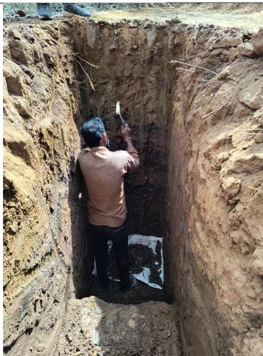
Photo. 10.5 Photograph showing sampling in progress at Pit No- 37 near Meghpar village.
