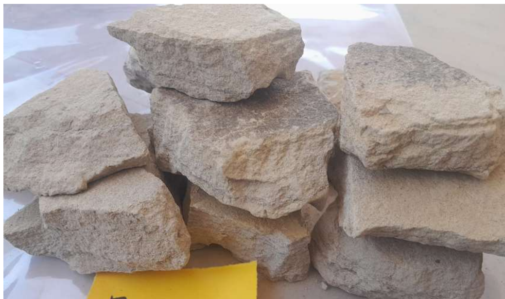
Photo 7.13 Photograph showing Bedrock sample of glauconite AW-04 (5.13% K 2 O) (23°37'04.8"N 68°59'20.1"E)
