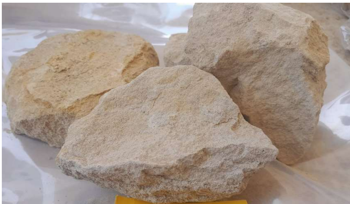
Photo 7.12 Photograph showing Bedrock sample of glauconite AW-15 (6.03% K 2 O) (23°35'16.0"N 68°57'49.2"E)
