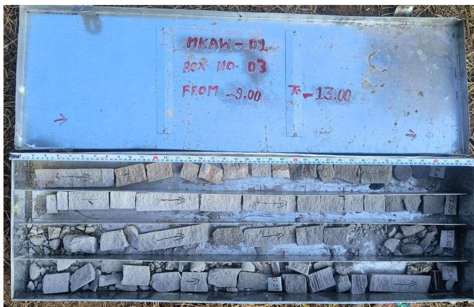
Photo-13.5 Photograph showing the half spitted cores of Borehole No-MKAW-01 of Ambara West Block
