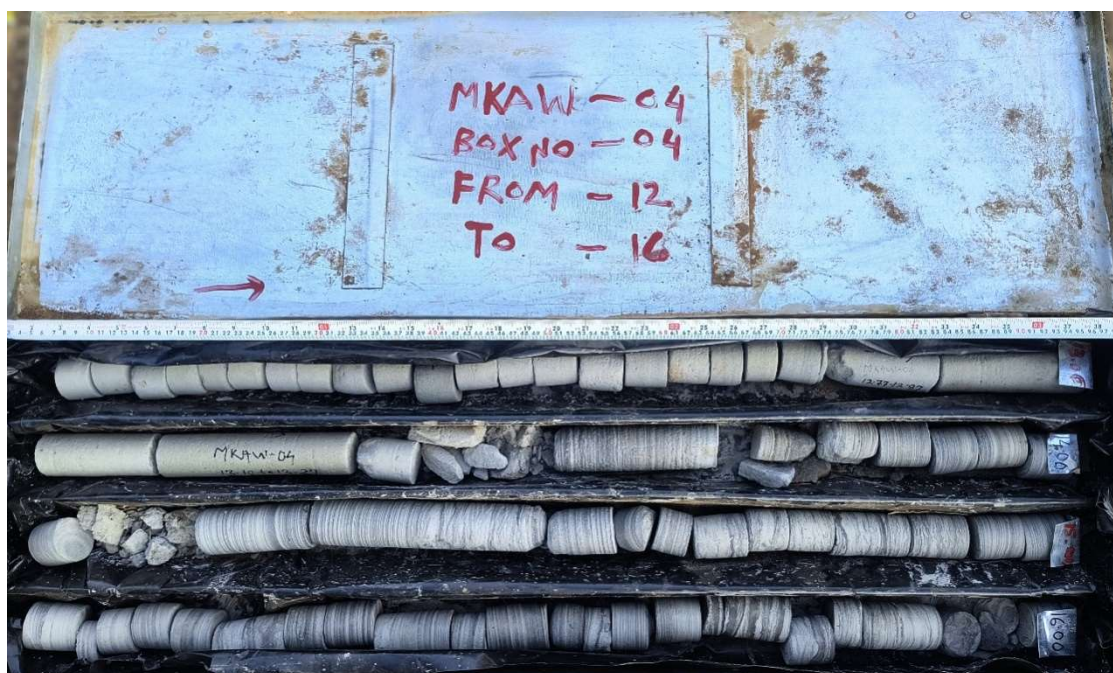
Photo 7.14 Photograph showing glauconite & Alternate band of glauconite horizons (Sandstone and Shale) in Borehole no- MKAW-04 (Depth-12.00m to 16.00m).
