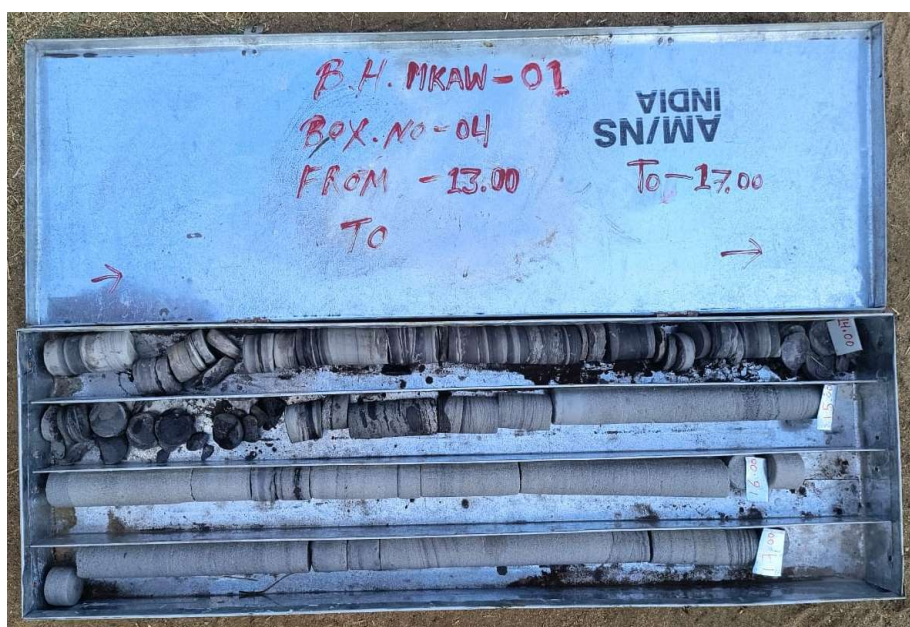
Photo-13.4 Photograph showing the recovered cores of Borehole No-MKAW-01 of Ambara West Block
